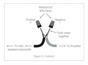
IMPORTANT: BE SURE NOT TO LET ANY STRAY '+' & '-' STRANDS TOUCH EACH OTHER. TOUCHING STRANDS CAN CAUSE A SHORT-CIRCUIT THAT COULD DAMAGE YOUR AMPLIFIER AND DEGRADE SOUND QUALITY.
