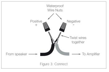
IMPORTANT: BE SURE NOT TO LET ANY STRAY '+' & '-' STRANDS TOUCH EACH OTHER. TOUCHING STRANDS CAN CAUSE A SHORT-CIRCUIT THAT COULD DAMAGE YOUR AMPLIFIER AND DEGRADE SOUND QUALITY.
