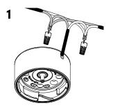
Connect the 70V wire run to the mount's pigtail using the included silicon wire nuts.
