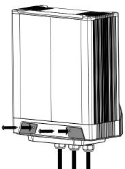
Rotate the MB1 so it stands vertically in the mount, allowing the wires to hang down. Screw the MB1 into the mount by hand.
